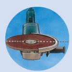
Make sure that the DCD surface and the mounting nut are in the same plane, after mounting.
