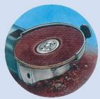
Never stop a machine by placing the wheel on the ground. Always place machine in proper stand or in an upright position.
