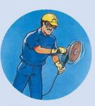
Allow the DCD to run at least for a minute before actual grinding, holding the machine away from body.
