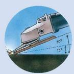
While operating, hold DCD at 15° - 30° to the work surface, for the best results.
