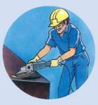
Do not apply excessive pressure while grinding (Recommended pressure 8-10 kg)
