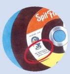
Ensure that the rated wheel RPM is in line with the machine RPM.
