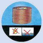
Store the DCD's one above the other, away from oil and moisture/water and in original packing.
